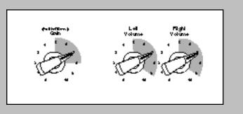
For tones that emphasize the Class "A" characteristics of the power amps, keep the Gain in Normal mode (pushed in) and set it below 5. Dial in some power amp distortion by setting the Volume controls above 5. Pushing the power amps this way creates a throaty quality you'll also notice that the tone controls are very responsive when the amp is used this way.
